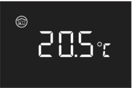
Floor heating shut down
